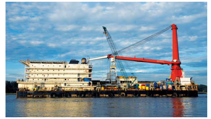
Derrick Lay Barge “Enterprise 3”
